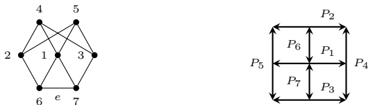
FIGURE: A B_0 -CPG graph containing K_{3,3} as a minor (contract e ).
