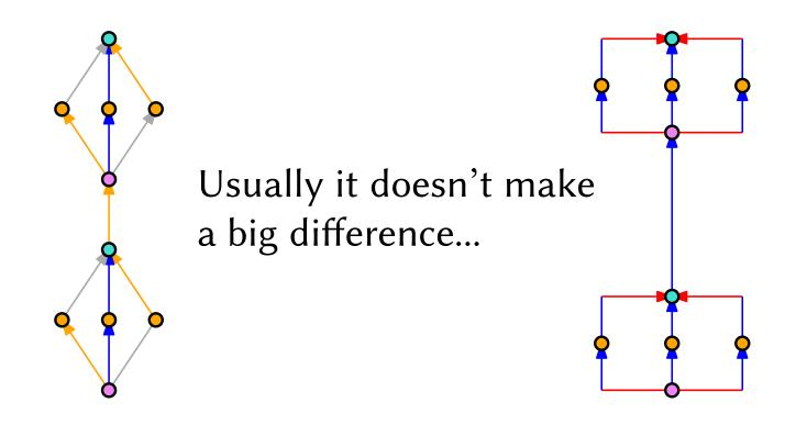
Every edge is drawn as a curve monotonically increasing in the *y*-direction
