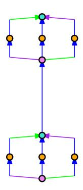
Every edge is drawn as a curve monotonically increasing in the *y*-direction
