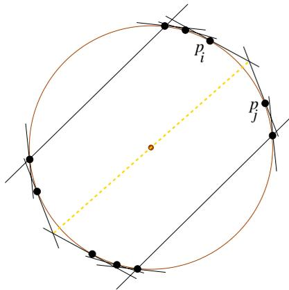
Figure 2: The diametral pair is reached in the intersection of the tangent lines through the two points  $p_i, p_j$  that define the maximum gap.
