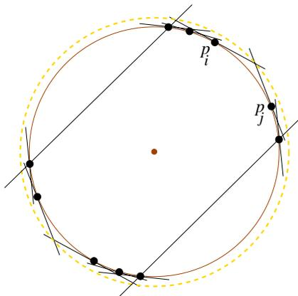
Figure 3: The minimum enclosing circle is determined by the points  $p_i$ ,  $p_j$  that define the maximum gap.
